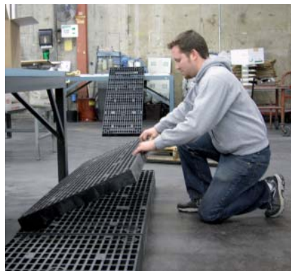
Use a portable work platform and adjust it to the height of the worker.
