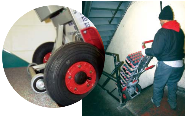
This is a powered two-wheel hand truck designed for climbing stairs.
