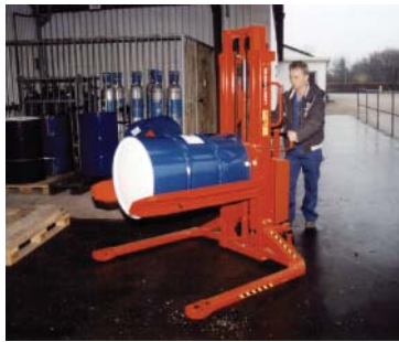
Stackers can be fitted with specially shaped forks to handle round or cylindrical containers.
